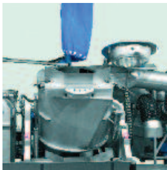
Front view loading – the cage tilts up to 70° upwards
